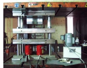
Fig. 3 Tool setup in the hydraulic press for forming the S-rail
