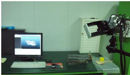
Fig. 7 Measurement of the 3-dimensional shape of the S-rail with 3D optical scanner
