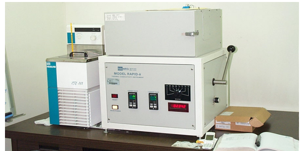
Fig. 5 Thermal conductivity measurement apparatus.
