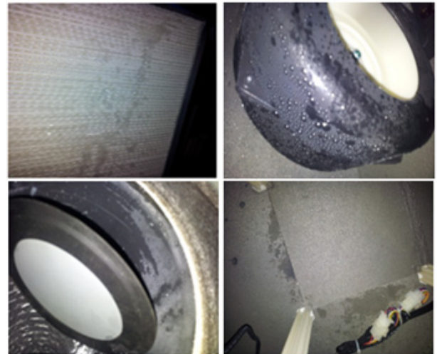
Fig. 4 Pictures of dew condensed parts.
