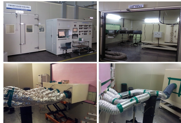
Fig. 3 Performance test facility of a heat recovery ventilator.
