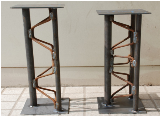
Fig. 4. Original (left) and reformed lattice girders used for the compression test
