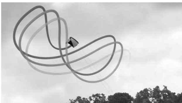
The system developed at Langley flies a kite in a figure-8 pattern to power a generator on the ground (Photo: NASA)
