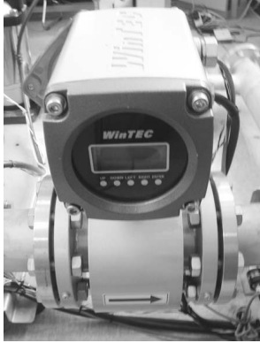
Fig. 2 Photo of flow meter
