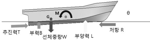
Fig. 5 Force Diagram in Running Condition
