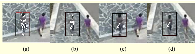
Fig. 4. (a), (b) Representation of pixels that have no similar color in background region; (c), (d) reference vector in 10th and 120th frames.
