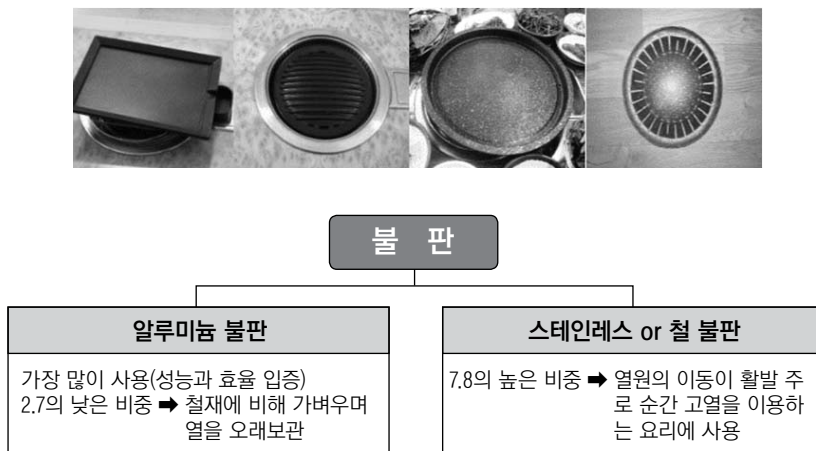
Fig. 2. Selection of the material for roasting plate
