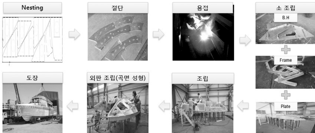
Fig. 1 Schematic construction process of Aluminum ship
