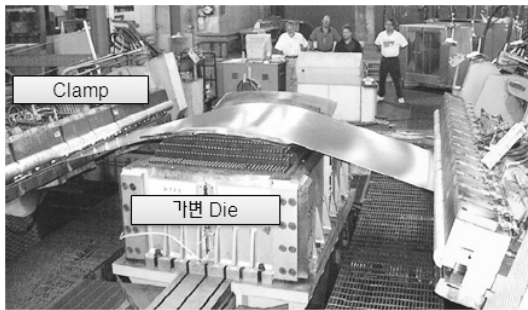
Fig. 8 Typical configuration of stretching forming (Boeing Co., Ltd.)
