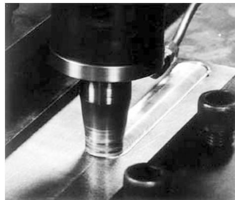
Fig. 6 FSW of Aluminum plates (Courtesy of Kawasaki Ind. Co.)
