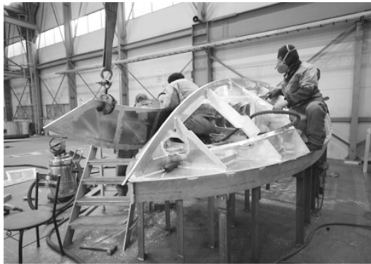
Fig. 7 Current practice of plate forming and assembly work
