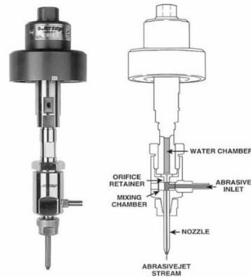
Fig. 2 Sectional view of a typical AWJ nozzle
