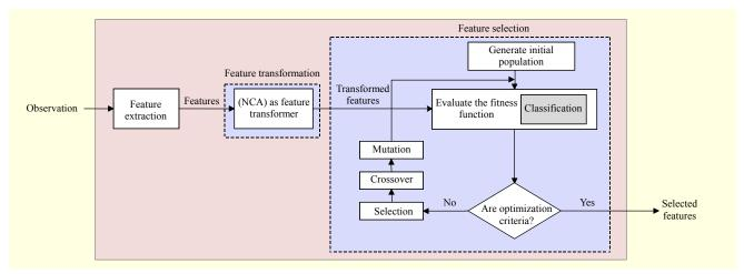
Fig. 1. Detailed block diagram of proposed method.
