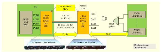
Fig. 2. 10/1G-EPON link structure using proposed hybrid-type PBEx.
