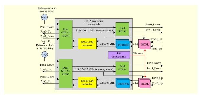
Fig. 5. Internal structure of FPGA for 3R-based signal regeneration [10].
