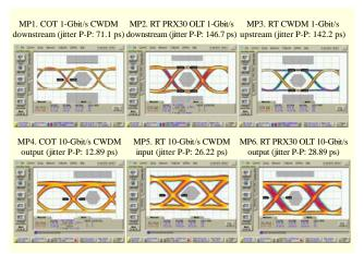
Fig. 7. Optical eye diagrams measured at each MP.
