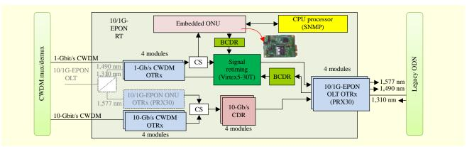
Fig. 4. Internal architecture of 10/1G-EPON RT.
