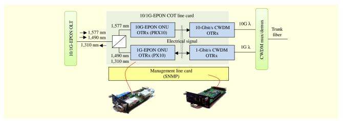
Fig. 3. Internal architecture of 10/1G-EPON COT line cards.
