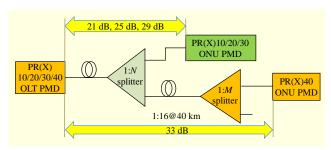
Fig. 1. 10G-EPON link structure suggested by IEEE 802.3 extended EPON study group [2], [3].
