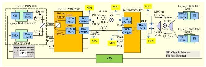
Fig. 6. Experimental setup for performance measurement of proposed hybrid-type 10/1G-EPON PBEx.
