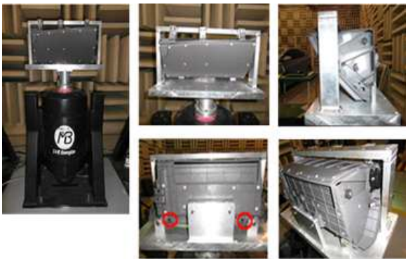
Fig. 8 Configuration of glove box FRF test
