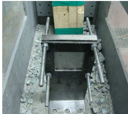
Fig. 6 Steel plate clamped in fixture frame
