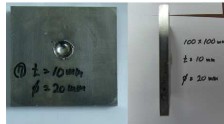
(b) Deformation : 6.1 mm
