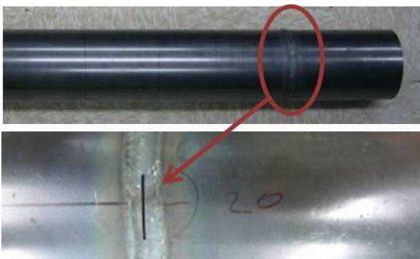
Fig. 3 Pictures of a pipe specimen and 20mm notch in welded zone
