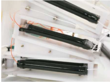
Fig. 8 Linear actuator in artificial muscle hand
