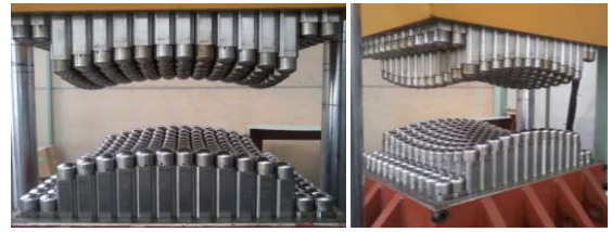
(a) Flexible die adjusted for saddle-type plate forming
