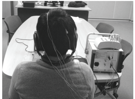
Fig. 7 Measurement of EEG on the measurement with 8ch electrodes
