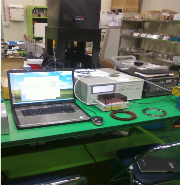
Fig. 3 Experimental set for measuring BH curve
