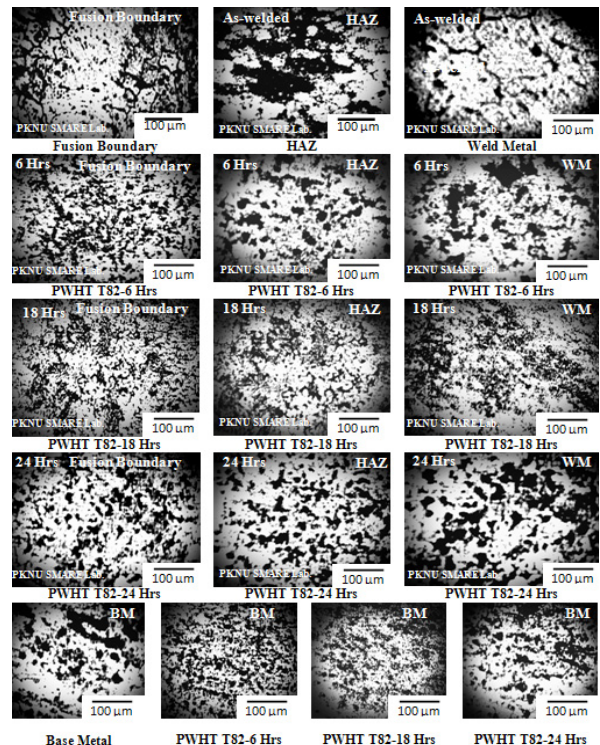
Fig. 9 Optical micrographs of As-welded and PWHT-T82 specimens for variety of aging
