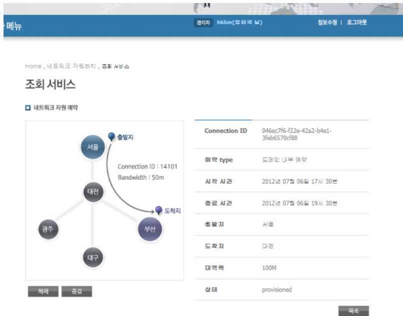
Fig. 13. GUI for Release or Termination Service from a Service of Provisioned Status
