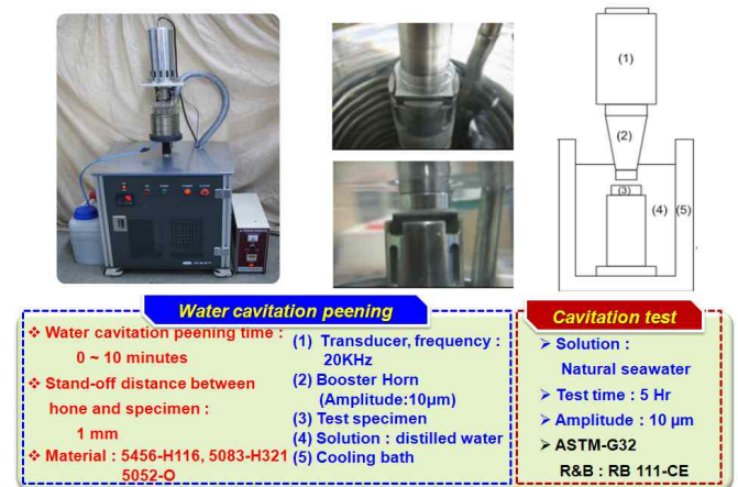
Fig. 1. Schematic diagram and apparatus for water cavitation peening in the distilled water and cavitation test in sea water.
