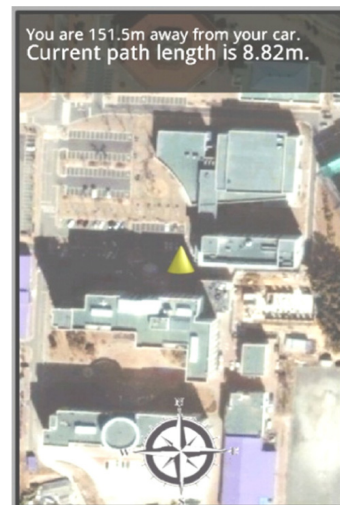
(Figure 7b) Based on the calculated step length of the user, the distance to be travelled towards the destination can be determined.
