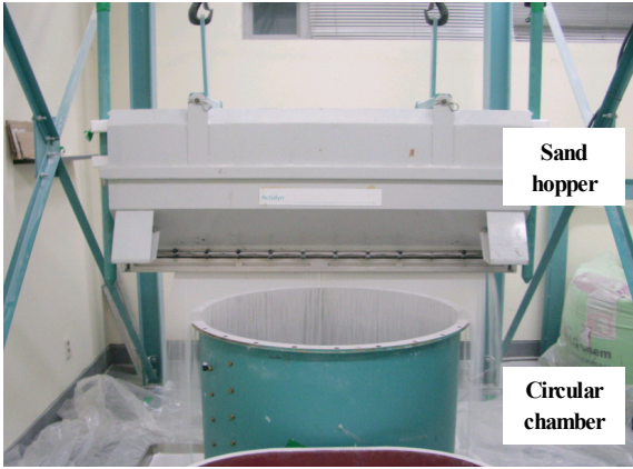
Fig. 4. Sand specimens with raining method with a sand diffuser
