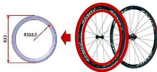
Fig. 2 Wheel geometry and 3D modeling.
