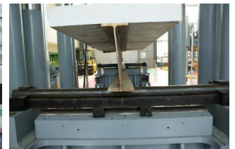
Fig. 16 Lateral buckling of H-composite beam
