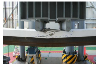
Fig. 15 Concrete slab collapse
