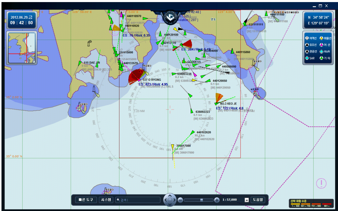
Figure 3. Computer monitor snapshot for maritime risk visualization system using final risk evaluation model
