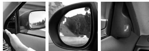
Fig. 4 Warning signal device
