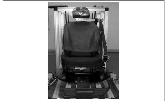
Fig. 10 Installation of pressure sensors on the headrest, and on the backseat
