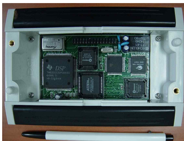
Fig. 2. Intelligent master controller based on LonWorks network
