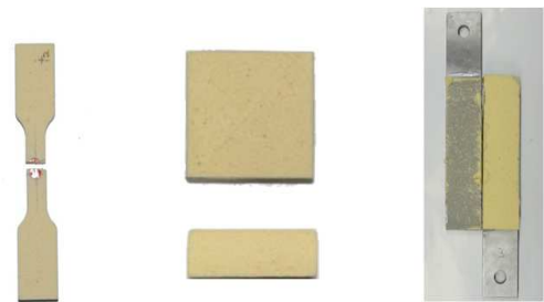
(a) Tensile failure mode (b) Compression failure mode (c) Shear failure mode
