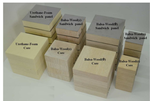
Fig. 6 Core materials and sandwich panel specimens for low-velocity impact test
