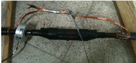
Fig. 3. Concept of the cable system for experiments and PD measurement
