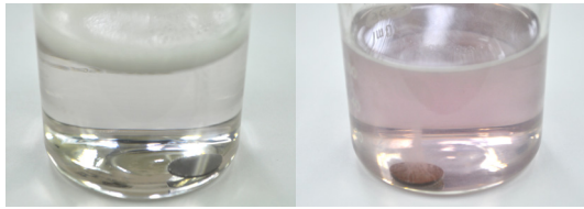
Fig. 3 Discoloration of propellant after material compatibility test (Left : Inconel 625, Right : Hastelloy C276)
