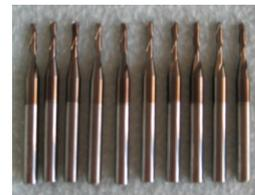
**Fig. 2 Plasma source ion implanted tungsten carbide endmill**
