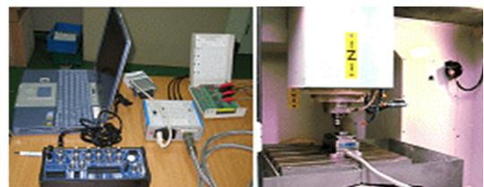
**Fig. 3 Experimental equipment of measurement cutting force by tool dynamometer**
