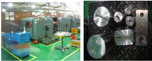
(a) Multi-stage former (b) dies
