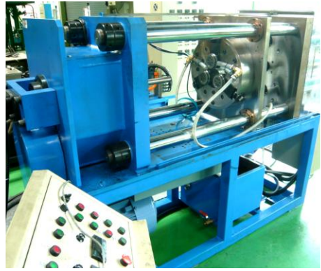
Fig. 1 Photograph of tube spinning equipment
