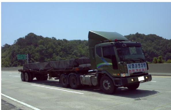
Fig. 4(b) Scene of Test running for weighing in Motion Axle Loads on Main Lanes of the Expressway
