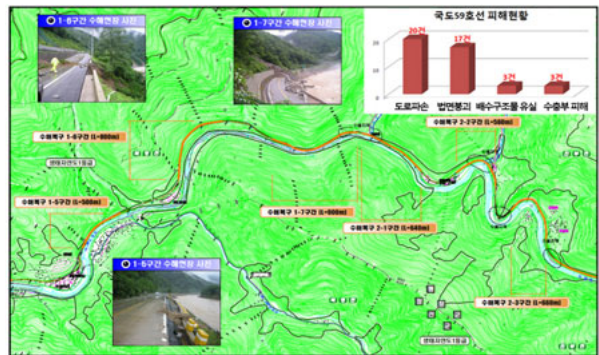
Fig. 11 Test-Bed Route(Natl. 59) Damage Drawing
