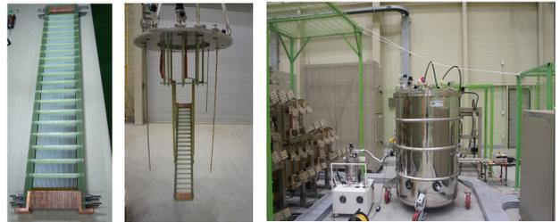
Fig. 8. SFCL unit module and experiment setup.
