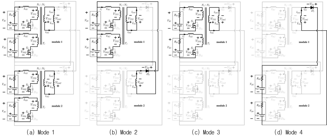
Fig. 2 Operating modes of the proposed modularized charge equalizer
