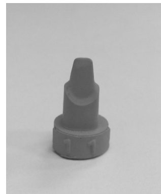
Fig. 2. Stone abutment model
