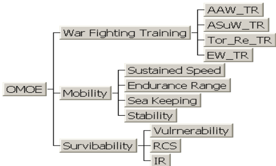
<Figure 5> OMOE breakdown structure
