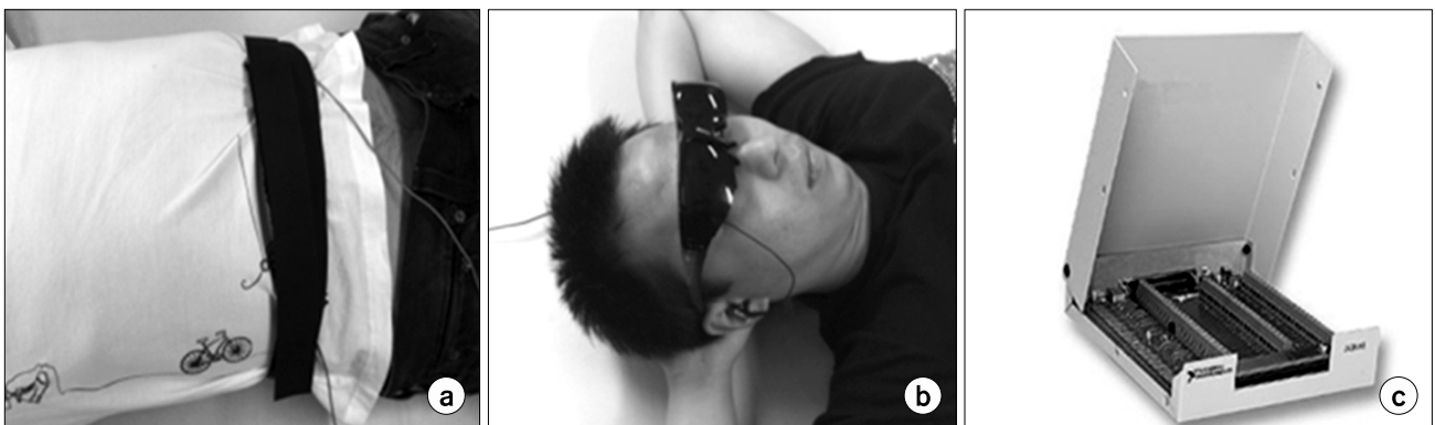
Fig. 1. Patient set-up to acquire respiratory signals using in-house developed belt type sensor (a), head mounted displayer (b) and SCB-668 DAQ card (c).
