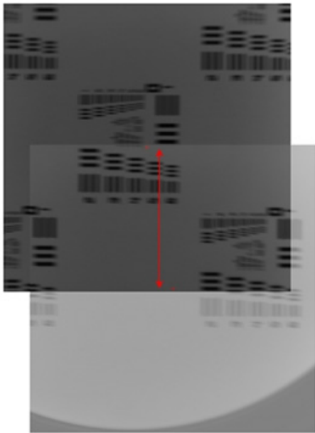
Fig. 11. Test result : displacement of #3 frame
