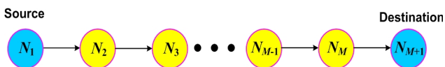
Fig. 1. An M -hop route from the source N_1 to the destination N_{M+1} .
