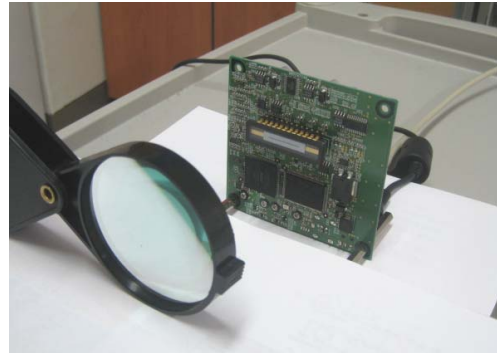
Fig. 2. Visible light communication receiver part using an image sensor, a driver circuit, and a lens.
