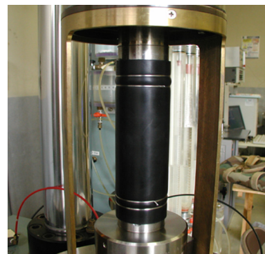
(c) 2 mm thickness of membrane for specimens
