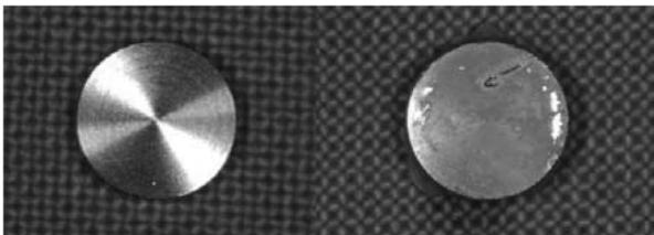
**Fig. 2.** Titanium disk used in biofilm formation. After disk preparation (left) and biofilm formation (right).
