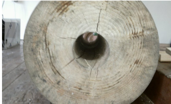
Fig. 6. A photo for crack development during pre-cracking.
