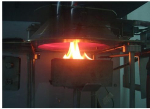
Photo. 2. Cone calorimeter test of fire retardant treated wood.
